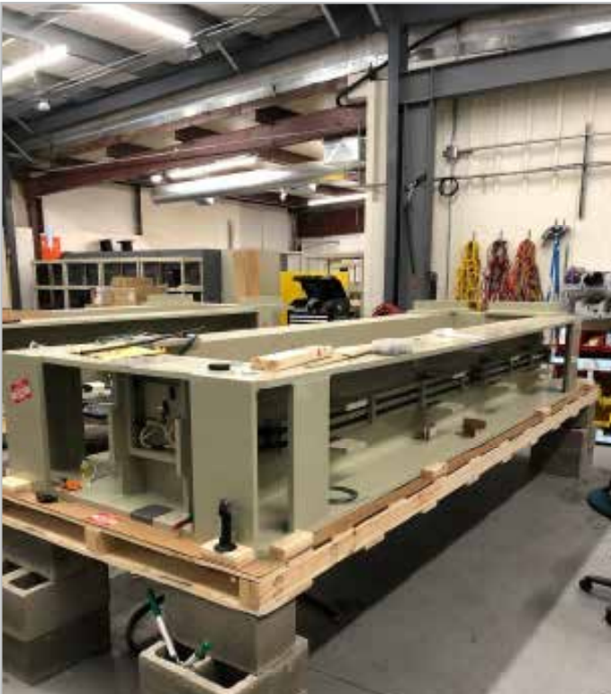
Figure 2. Washington Shore serpentine weir replacement antennas under construction at the PTAGIS Kennewick Lab. Photo courtesy of PTAGIS Staff
