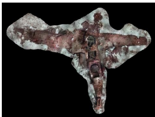
Figure 3.—Photomosaic of a WWII plane crash developed during surveys with the SeaBED AUV.
