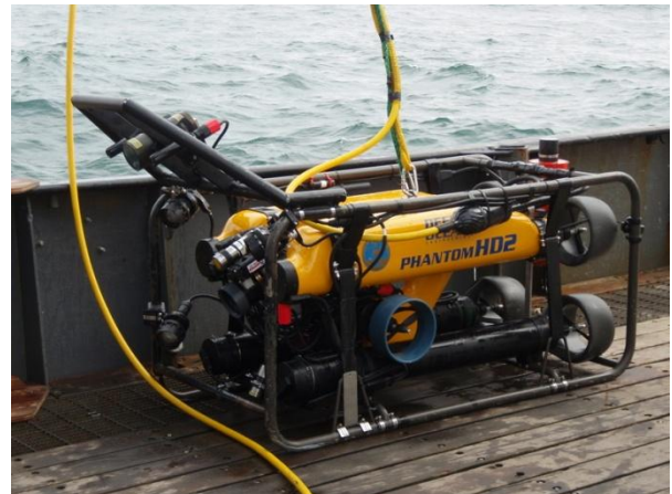
Figure 2. Buttercup showing forward and belly cameras. Not shown are stereo cameras and auxiliary light frame.
