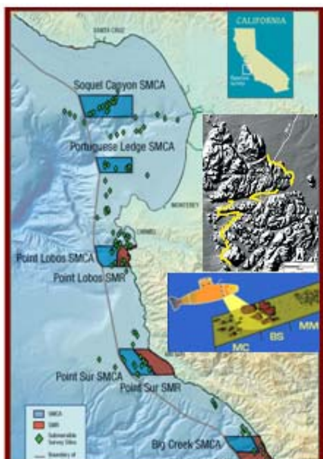
Figure 5: Survey sites in and out of MPAs off central CA. Top inset: Submersible transect over map of rock outcrop. Bottom inset: Schematic of habitat patches (mud, boulder, cobble, sand) along submersible
