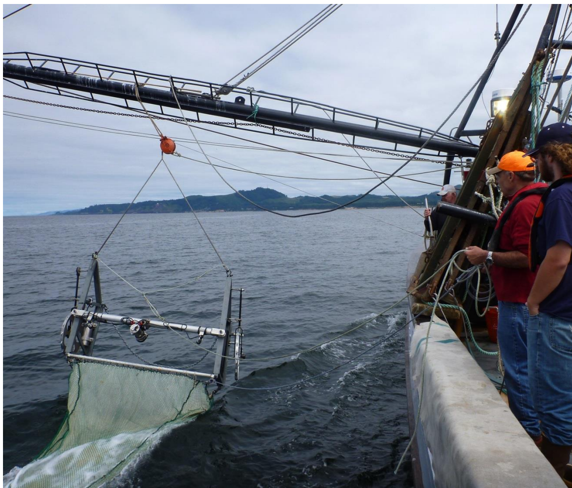
Figure 3. NMFS and PSMFC researchers and the crew of the F/V Miss Yvonne look on during a deployment of the beam trawl system equipped with HD camera and scaling lasers. F/V Miss Yvonne, off Newport OR, July 30 th 2012.
