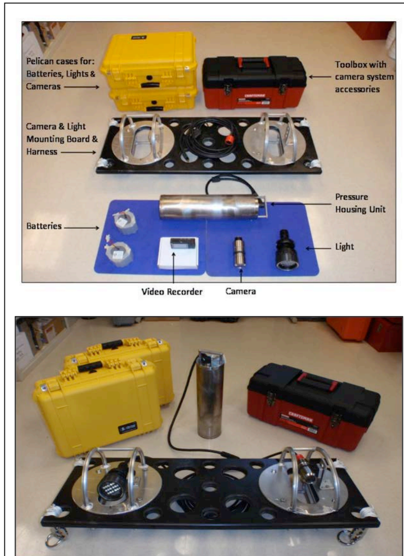
Figure 14. One of four autonomous direct observation video camera systems developed at the NWFSC.
