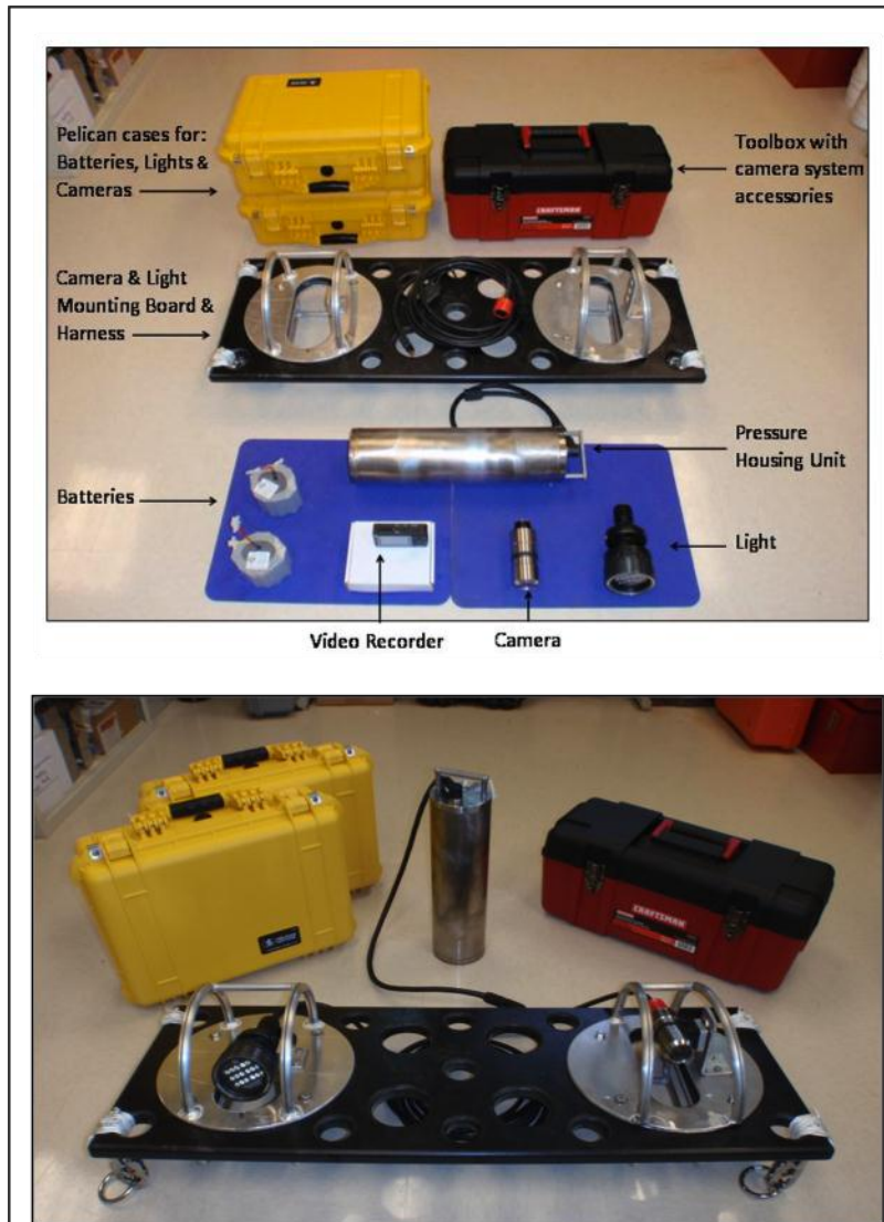
Figure 8. One of four autonomous direct observation video camera systems developed at the NWFSC.
