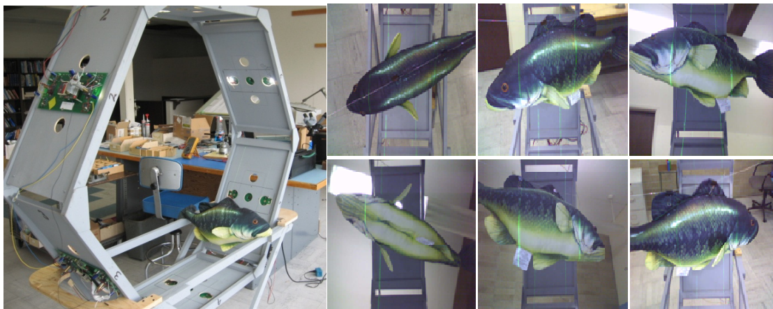
Figure 2. Figure illustrates the configuration of the QUOTAS prototype. A total of 6 camera units are activated in a group of 3 to sequentially illuminate the sample volume bounded by the
