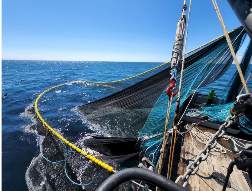
Figure 19: Purse seine being hauled in along the starboard side of the Lisa Marie .
