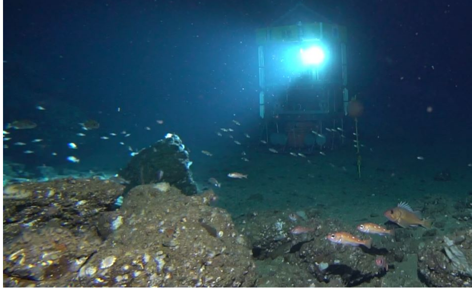
Figure 4. Top image: A surveillance platform resting on the seafloor. Lower level contains the computers and batteries, middle level contains the stereo cameras and other instrumentation, and upper level houses the DIDSON sonars and the strobe for the cameras. Image was taken from the manned submersible. For reference, the green lasers are 20 cm apart. Bottom image: The surveillance platform (with strobe flashing) as viewed from the MLML drop camera.
