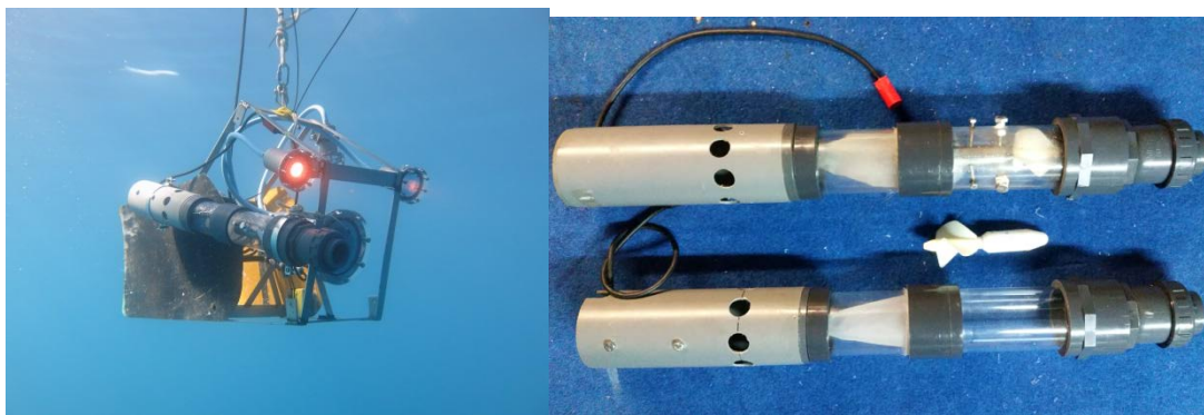
Figure 3. Plankton pump and deployment system with camera and lights. Images courtesy of ShelfReCover
