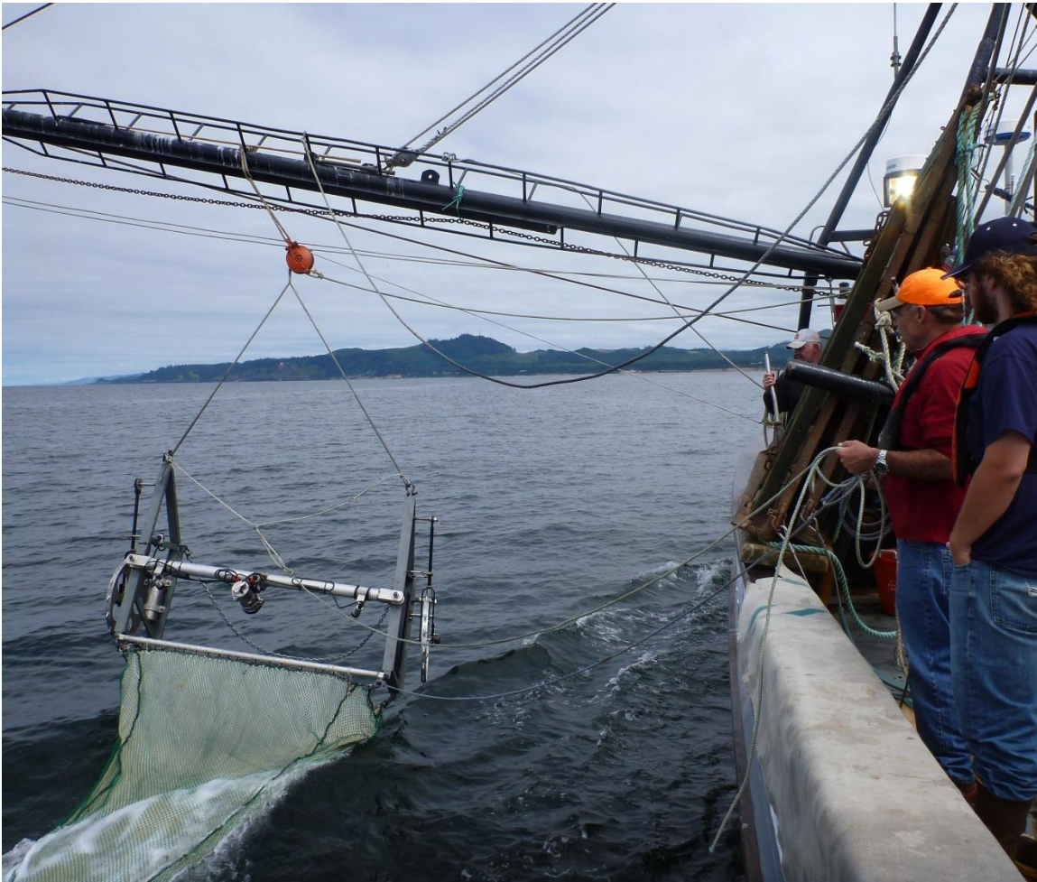
Figure 2. NMFS and PSMFC researchers and the crew of the F/V Miss Yvonne look on during a deployment of the beam trawl system equipped with HD camera and scaling lasers. F/V Miss Yvonne, off Newport OR, July 30 th 2012.
