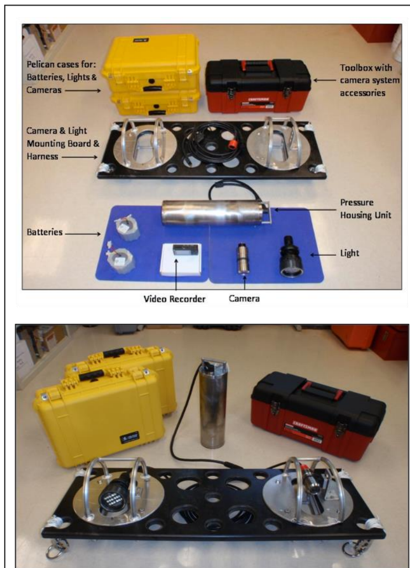
Figure 14. One of four autonomous direct observation video camera systems developed at the NWFSC.
