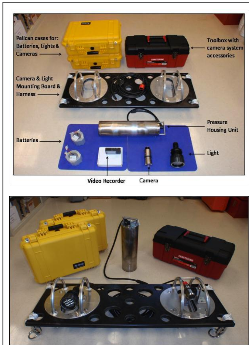
Figure 8. One of four autonomous direct observation video camera systems developed at the NWFSC.
