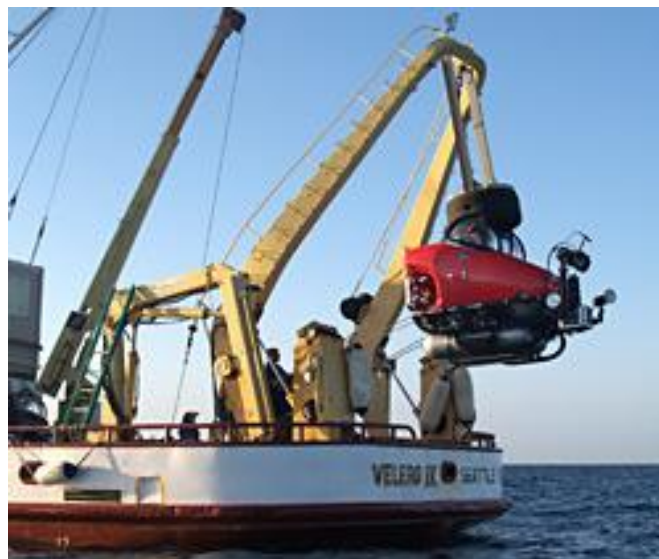
Figure D1. Two-person submersible Dual Deepworker being launched off the F/V Velero during a survey of demersal fishes and habitats on the Footprint seamount in the Southern California Bight.
