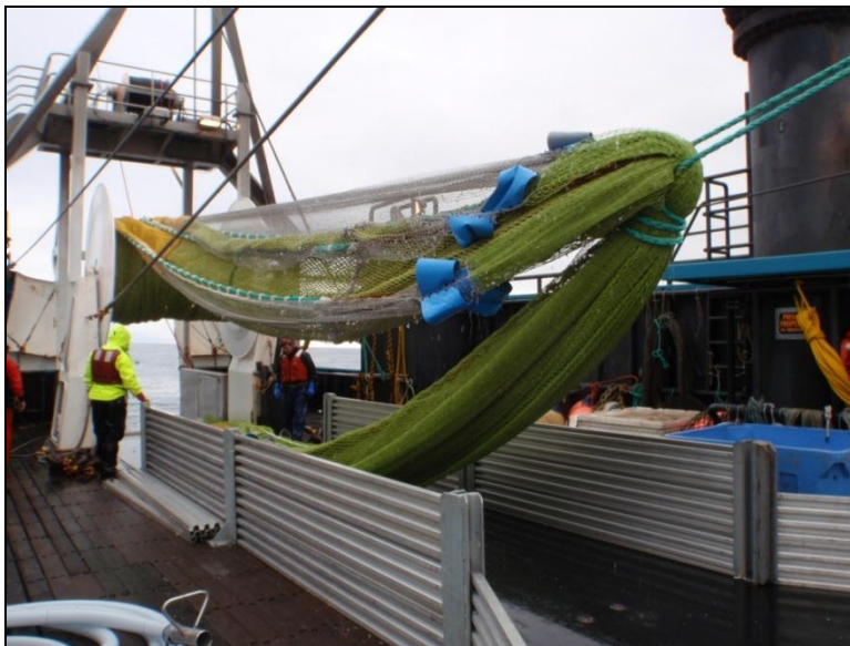
Figure 18. Bycatch Reduction Device and recapture net being deployed aboard a commercial fishing vessel off Washington during July 2011.
