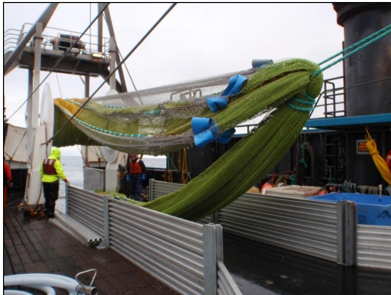
Figure 19. Bycatch Reduction Device and recapture net being deployed aboard a commercial fishing vessel off Washington during July 2011. Blue objects encircling recapture net are kites used to hydrodynamically open the net.
