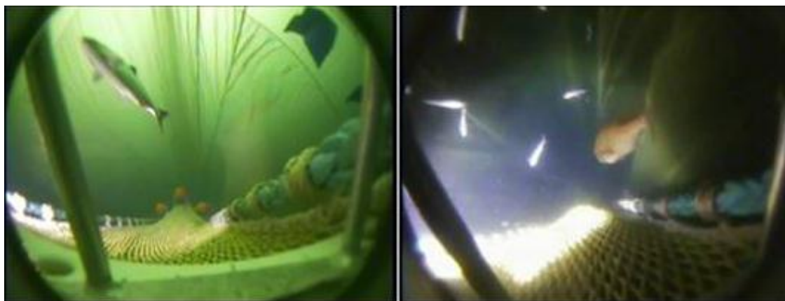
Figure 20. Video frame grabs showing Chinook salmon (left image), and widow rockfish with Pacific hake (right image) swimming inside the recapture net surrounding the BRD.
