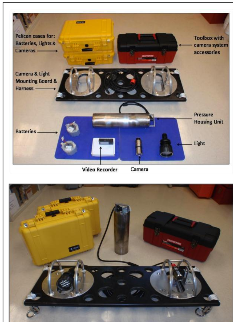
Figure 23. One of five autonomous direct observation video camera systems developed at the NWFSC.
