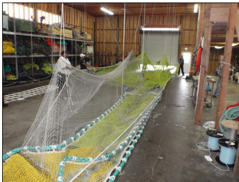
Figure 17. Recapture net under construction and integration with bycatch reduction device in a net loft in Newport, Oregon.
