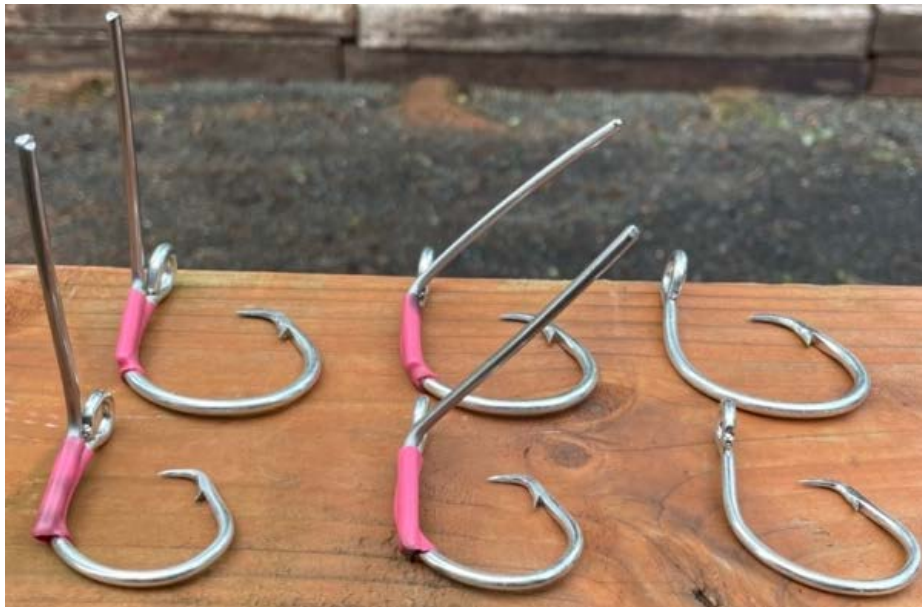
Figure. 1. Images of 16/0 (bottom row) and 18/0 hooks (top row) with 90° appendage (left), 45° appendage (middle), and no appendage (right).
