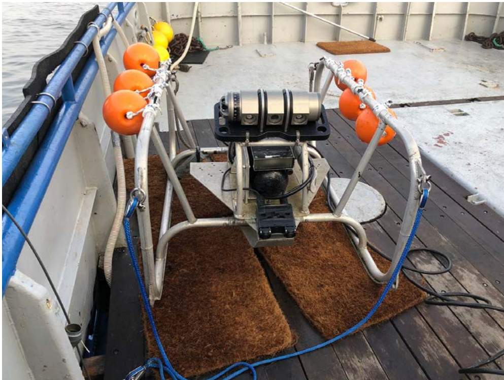
Figure 1. Image of the sled to be towed to observe trawl-seafloor interactions.
