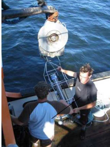
Figure 4: CTD being deployed using a crab block
