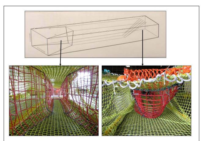
Figure 1. Schematic 3D view of a Pacific halibut flexible sorting grate excluder (top); aft looking view of the forward portion of the excluder where fish enter and encounter the device (bottom left); forward view of the aft end of the excluder where fish larger than the sorting grate openings would be guided and excluded from the trawl out on the top panel (bottom right). Image and design is courtesy of Dantrawl, Inc., Seattle, WA.
