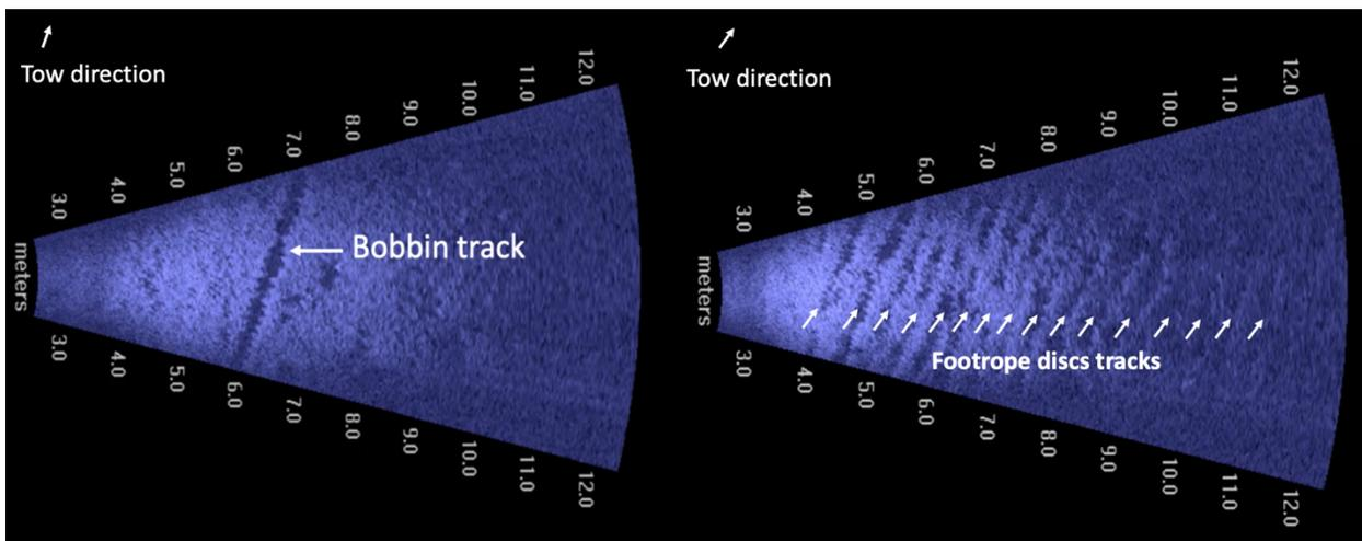
**Figure 7.** DIDSON imaging sonar frame grabs showing a bobbin track created by the elevated sweeps (left image), and an 8 m long section showing a portion of the tracks created by the footrope.
