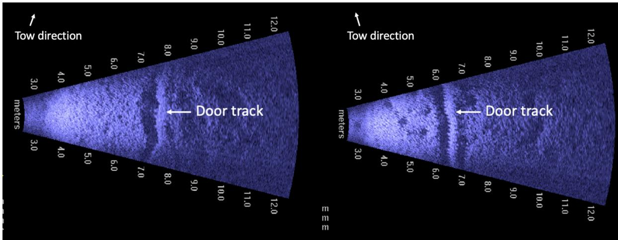
**Figure 6.** DIDSON imaging sonar frame grabs showing door tracks created by the conventional bottom door on two different tows.
