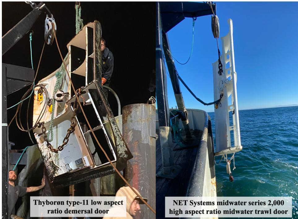
**Figure 1.** Image of the Thyborøn type-11 bottom trawl door (left image; size = 4.8 m<sup>2</sup>; weight = 995 kg) and a NET Systems midwater 2000 trawl door (right image; size = 4.5 m<sup>2</sup>; weight = 568 kg) used on the conventional and semi-pelagic trawl, respectively.
