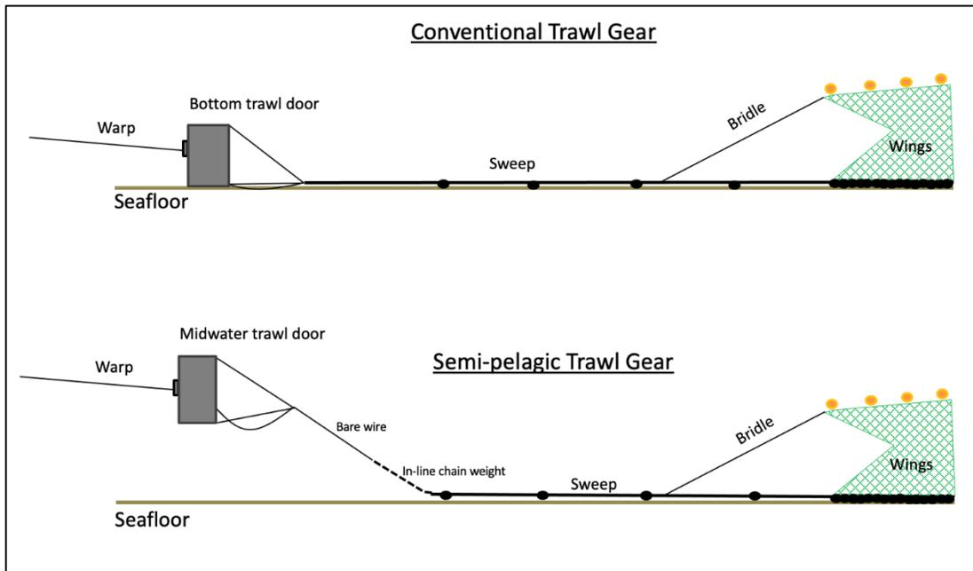
**Figure 2.** Schematic comparing conventional trawl gear rigged with bottom tending doors (top image) to semi-pelagic trawl gear rigged with midwater trawl doors (bottom image).
