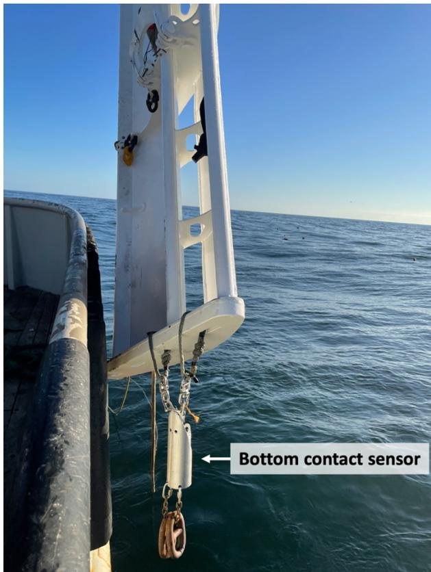
**Figure 3.** Image of a bottom contact sensor rigged to the semi-pelagic midwater trawl door.
