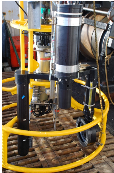
Figure 5. NWFSC Digital Video Plankton Recorder
