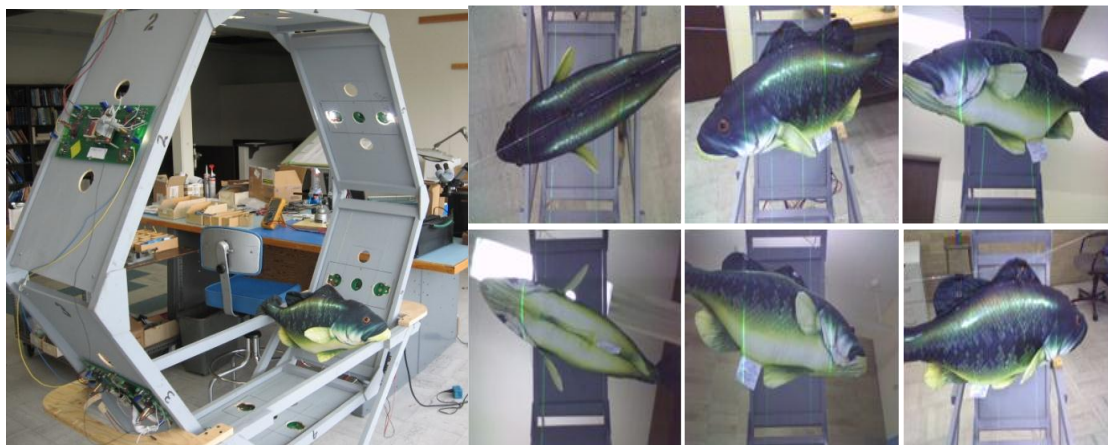
Figure 2. Figure illustrates the configuration of the QUOTAS prototype. A total of 6 camera units are activated in a group of 3 to sequentially illuminate the sample volume bounded by the ring frame. The laser pair on each camera is used to size the illuminated targets. The figure also illustrates one cycle of six images obtained from the prototype.
