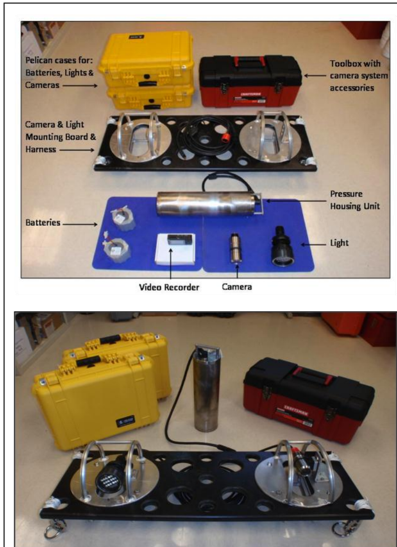
Figure 7. One of two autonomous direct observation video camera systems developed at the NWFSC with 2010 BREP funding.
