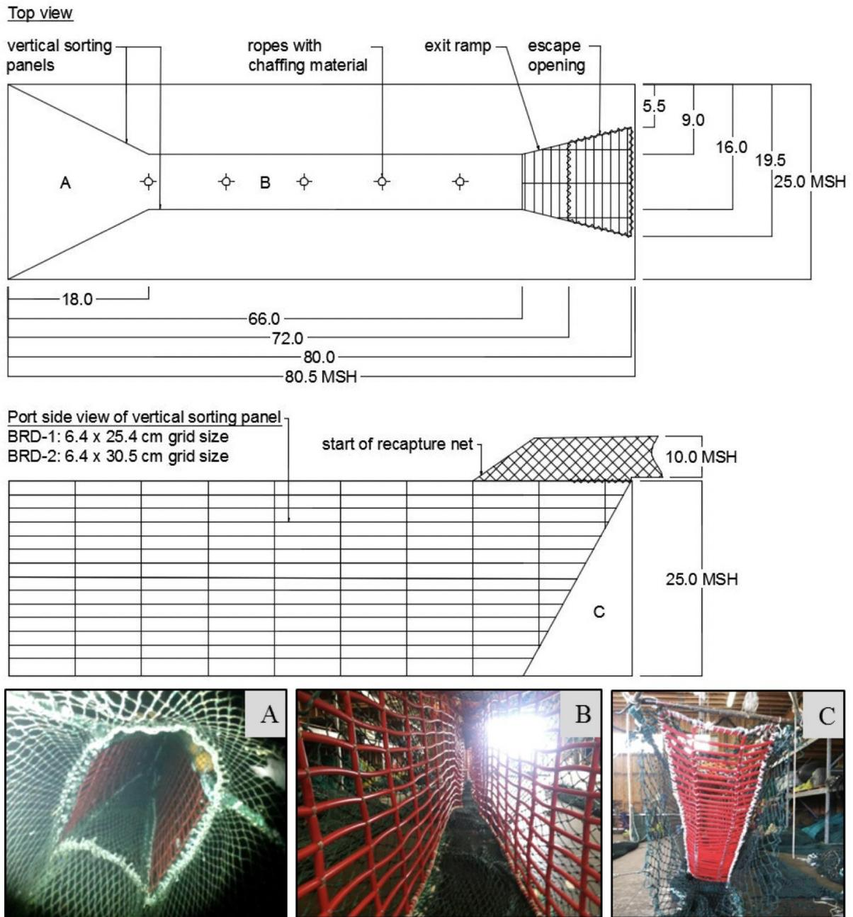
Figure 1. Schematic diagram (not to scale) of the flexible sorting grid general design tested (top). The only design difference between BRD-1 and -2 are the grid sizes. Aft view of the forward portion of the gear where fish enter and encounter the BRD (image A); aft view of the area between the two vertical sorting panels (image B); fore view of the upward-angled exit ramp (image C). MSH = meshes.
