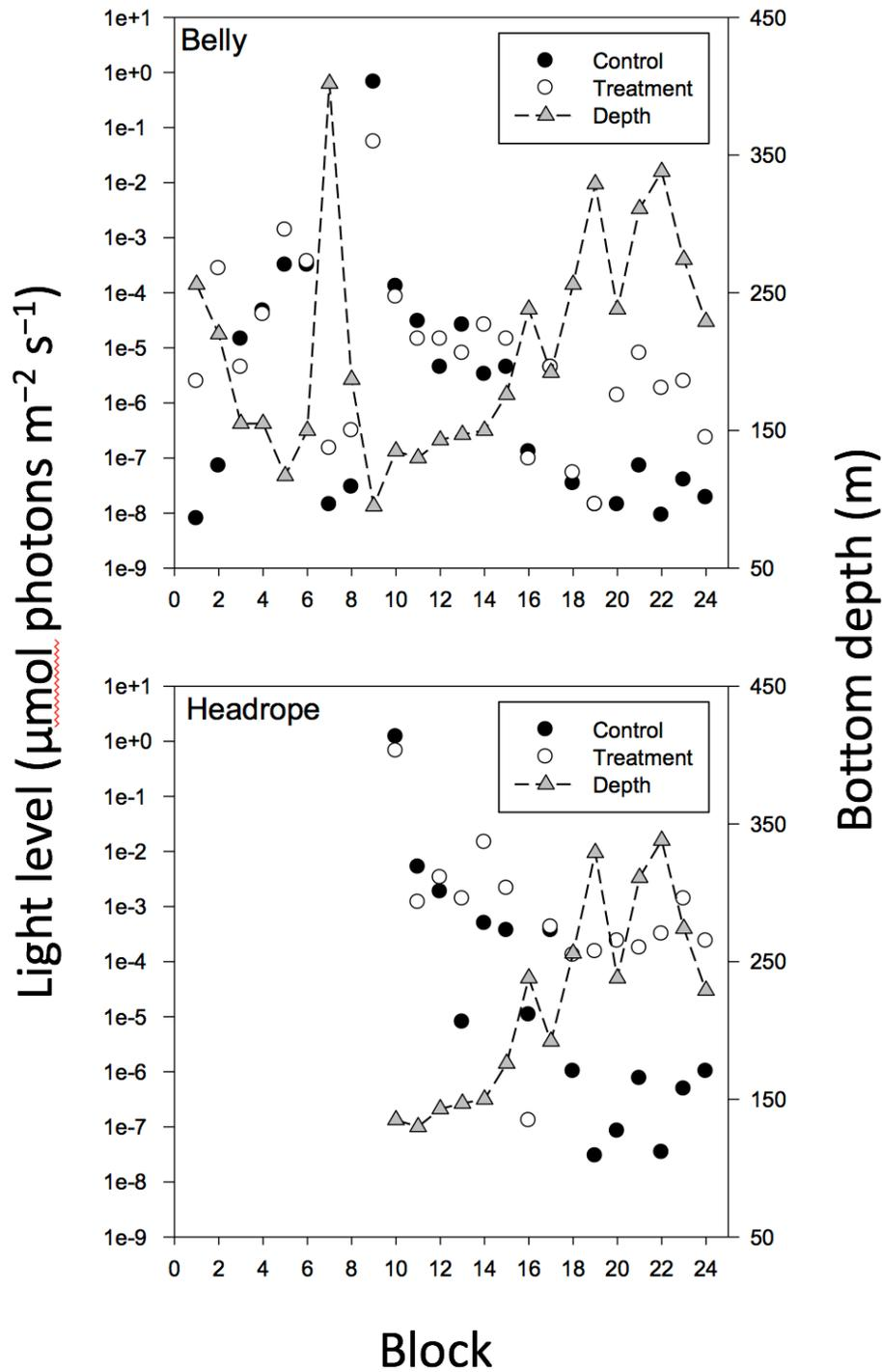
Figure 7. Mean light levels at the center of trawl belly and headrope and mean bottom fishing depths per block. Control = without LEDs; Treatment = with LEDs.
