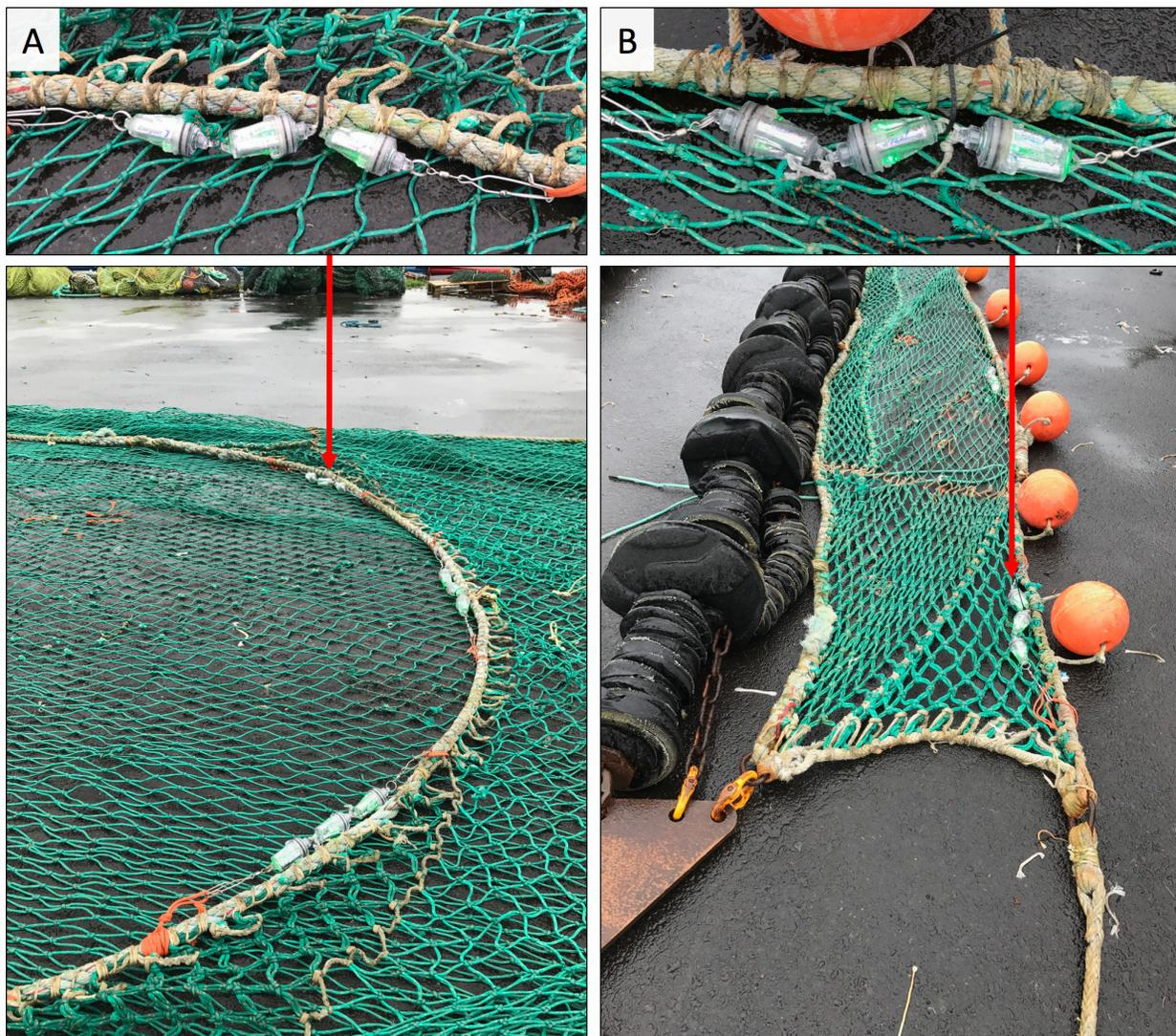
Figure 1. Image of an LED cluster attached near the center of the trawl headrope (A, starboard-side) and wing tip (B, port-side) and their orientation.
