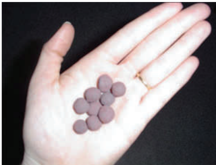
Taconite pellets - a typical example of non-toxic, non-hazardous dry cargo residue - can pose a significant concern if they are jettisoned in large amounts. (USCG photo)
