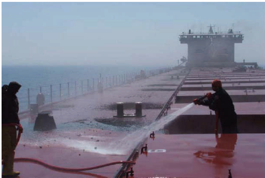
Deck washdown of coal residue after loading. (USCG photo)
