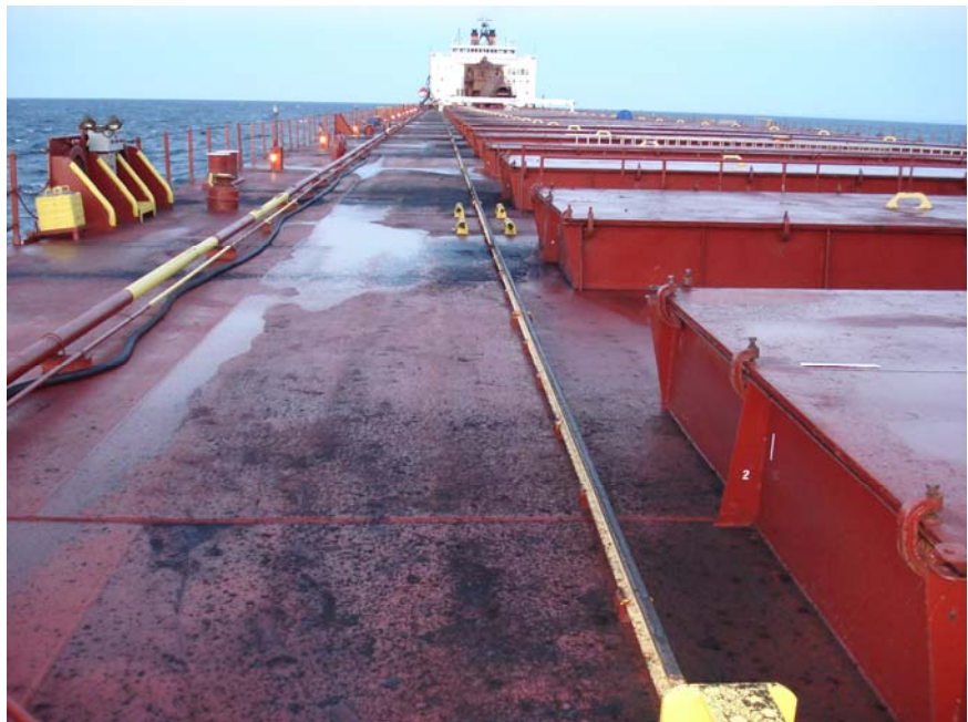
Cargo residue on deck after coal loading operation. (USCG photo)
